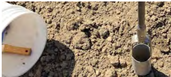
A 2.75-inch (7 cm) wide auger used for taking samples of the top 3 inches soil for bulk density analyses. Photo: Garrett Boudinot, Cornell
