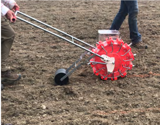
Seeding using a manual seeder for high-cannabinoid Cannabis. Photo: Savanna Shelnett, Cornell
