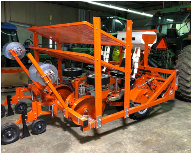
Transplanter machine allowing consistent space between plants and a better packing. Photo: Larry Smart, Cornell
