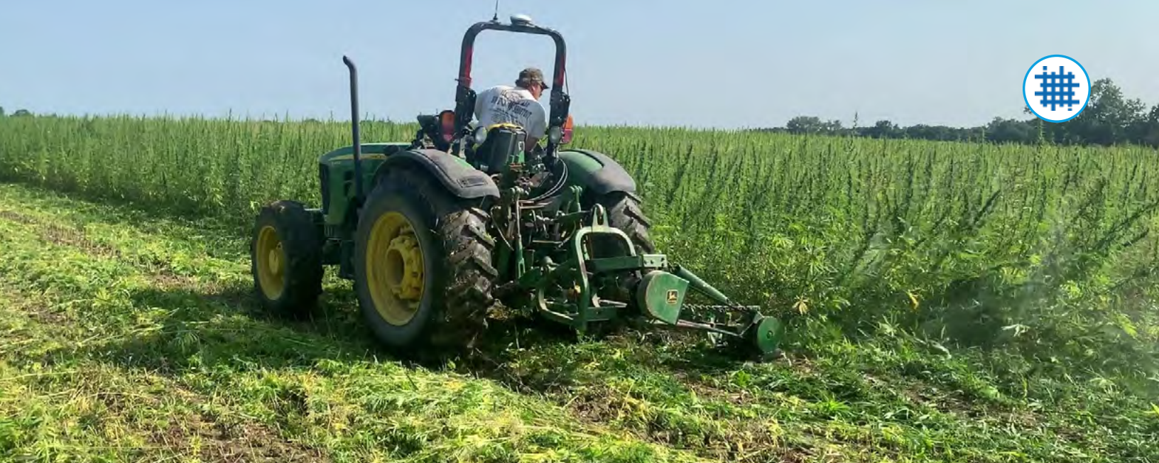
Fiber harvest using a sickle bar mower, Geneva, NY. Photo: Anthony Barraco III
