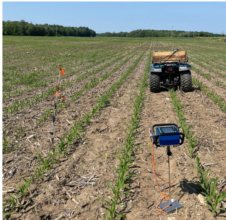
Digital penetrometer and related equipment used to collect soil compaction data in commercial farm fields.
