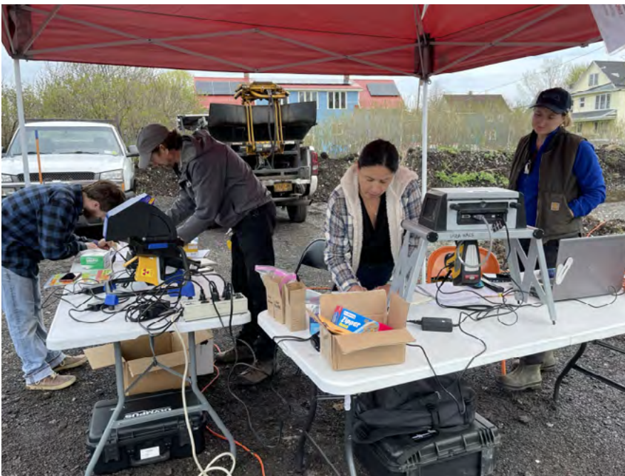
Soil health experts and technicians use specialized pXRF machine to screen community soil samples.
